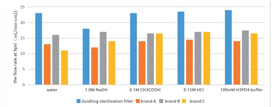
Membrane Flux of Sterilization Filters
