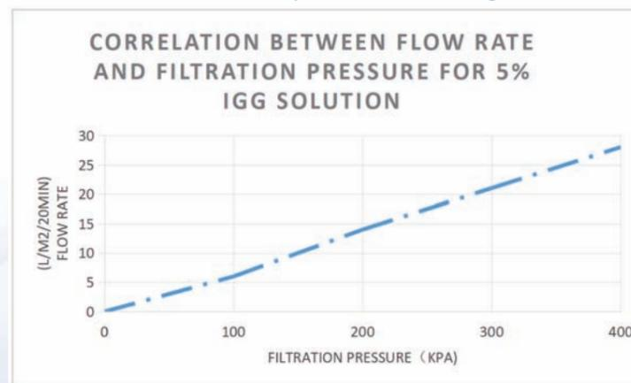
The flow rate is positively related to the filtration pressure, the higher the pressure, the faster the flow rate
