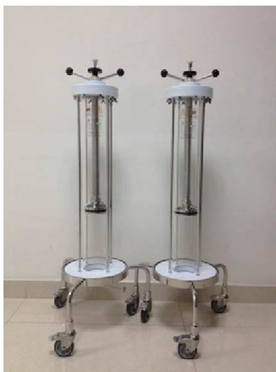
Appearance of chromatographic column ( Φ100 mm 、 Φ600 mm )
